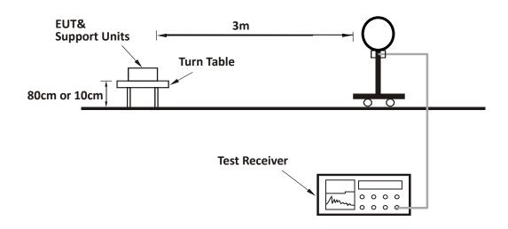
For Radiated emission 30MHz to 1GHz:
