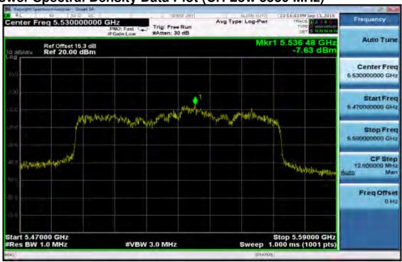
802.11ac VHT80, 5470~5725 MHz Peak Power Spectral Density Data Plot (CH High 5610 MHz)
