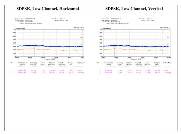
Note: The maximum output power mode and channel: 3EDR(8DPSK) mode \_ Low Channel was tested.
