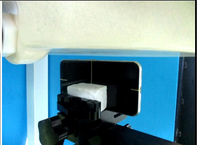
Right Side of EUT with 1.0 cm Gap
