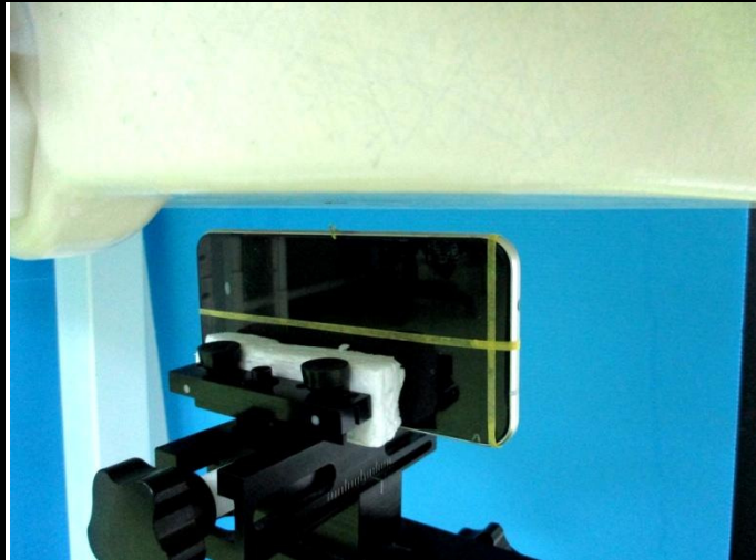
Left Side of EUT with 1.0 cm Gap
