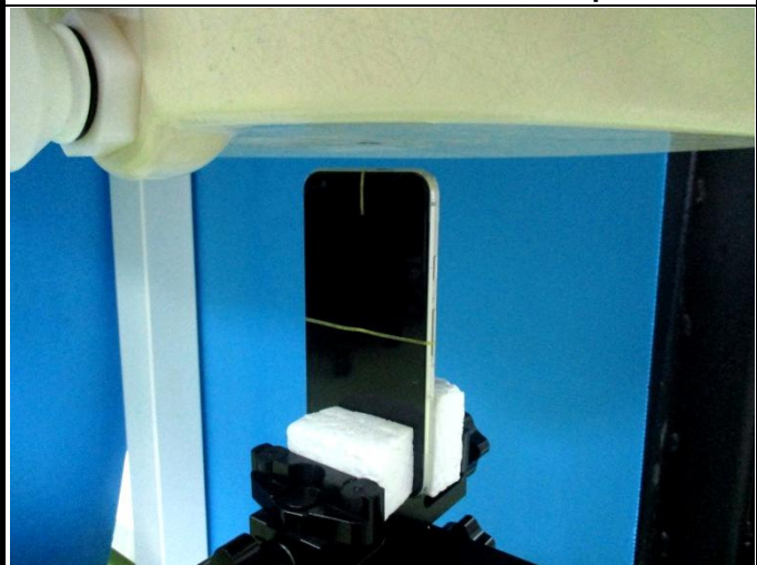
Top Side of EUT with 1.0 cm Gap
