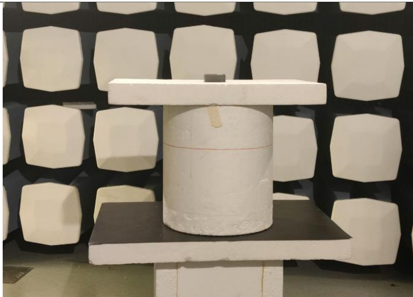
Picture 11, Radiated Spurious Emissions, EUT setup, TX 1 – 26 GHz
