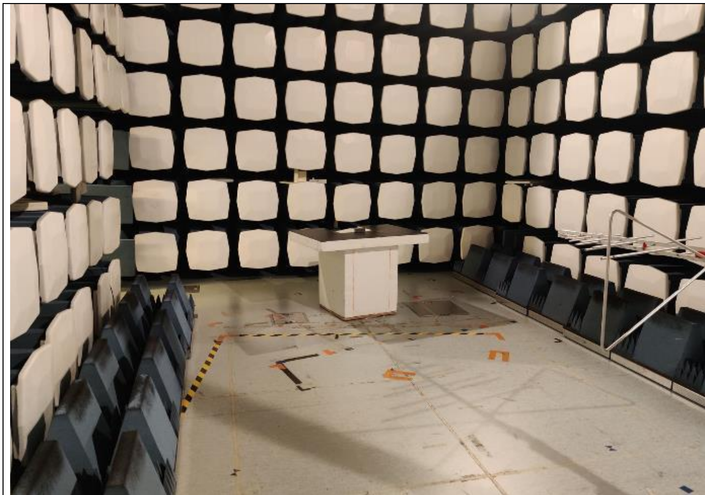
Picture 7, Radiated Spurious Emissions, common setup, TX and RX 30 - 1000 MHz
