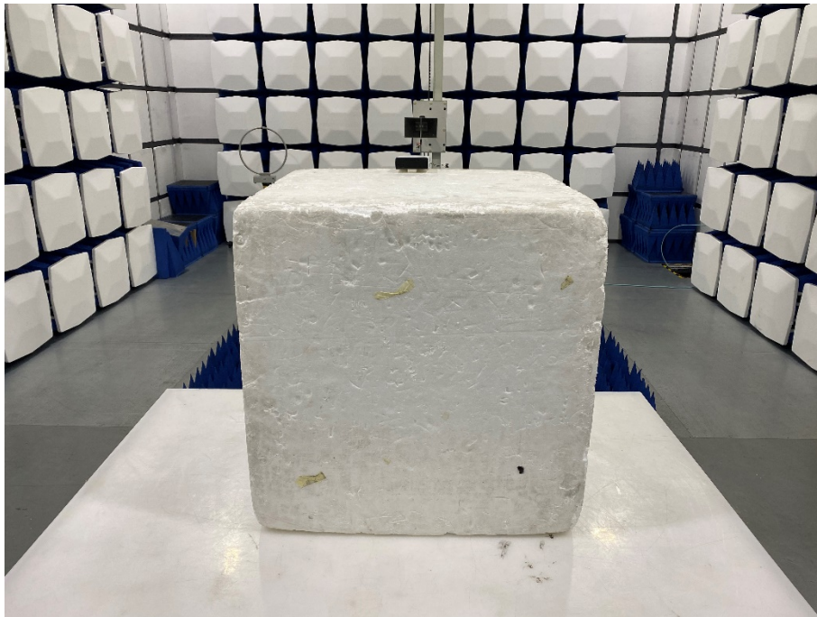
Photograph 3: Set-up for Radiated Spurious Emission, above 1GHz
