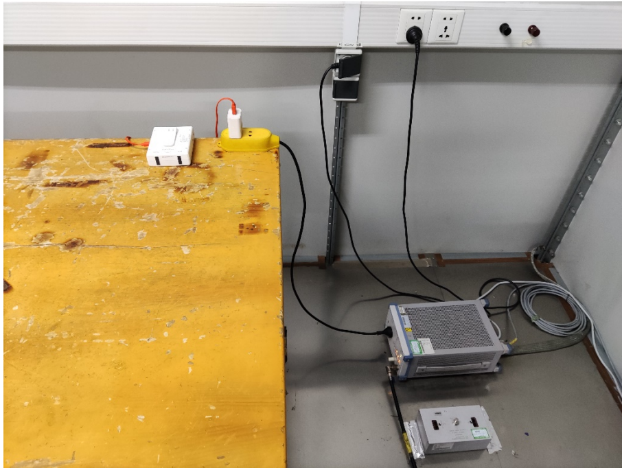
Photograph 1: Set-up for Conducted Emission on AC Mains
