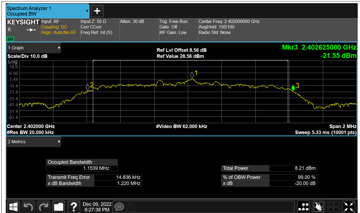
-20dB Bandwidth NVNT 3-DH1 2441MHz Ant1
