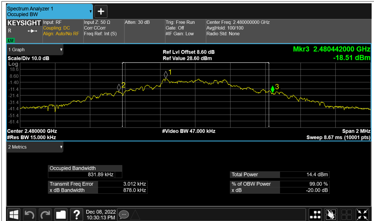
-20dB Bandwidth NVNT 2-DH1 2402MHz Ant1
