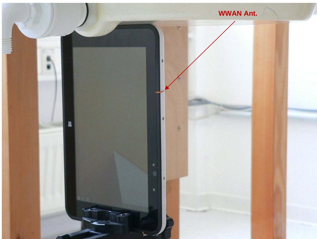
Fig. 23: Left edge of Inari8-3GAN-1, 0 mm distance, WWAN antenna, proximity sensor OFF.
