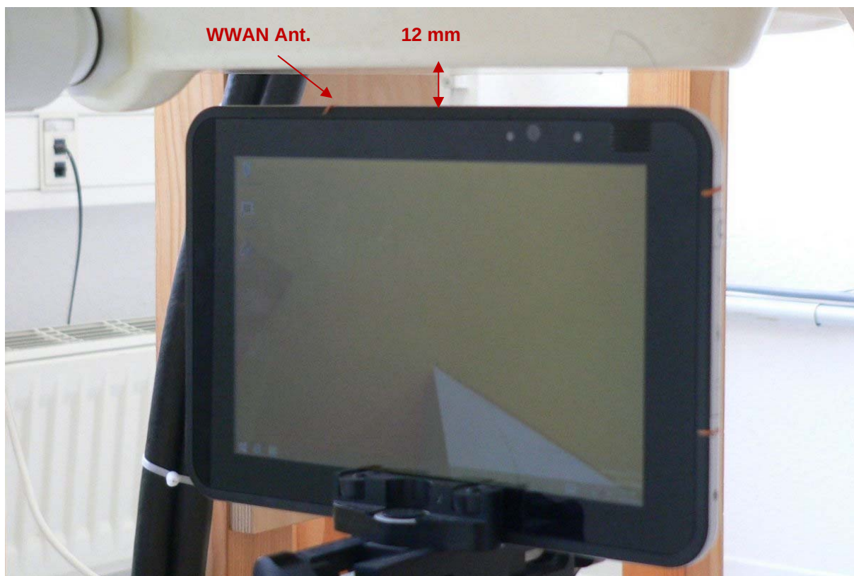
Fig. 22: Top edge of Inari8-3GAN-1, 12 mm distance, WWAN antenna, proximity sensor OFF.
