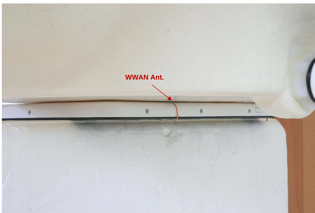
Fig. 24: Back side of Inari8-3GAN-1, 0 mm distance, WWAN antenna, proximity sensor ON.
