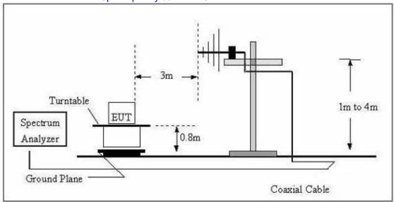
(C) Radiated Emission Test-Up Frequency Above 1GHz
