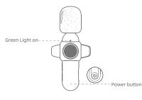
Last: Green light of both receiver and mic are always on ,means connected successfully. It's ready to record.
