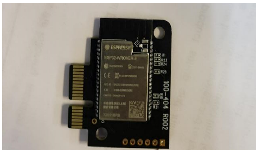
Figure 6. Wi-Fi Module (Pre-Certified) Removed from Enclosure
