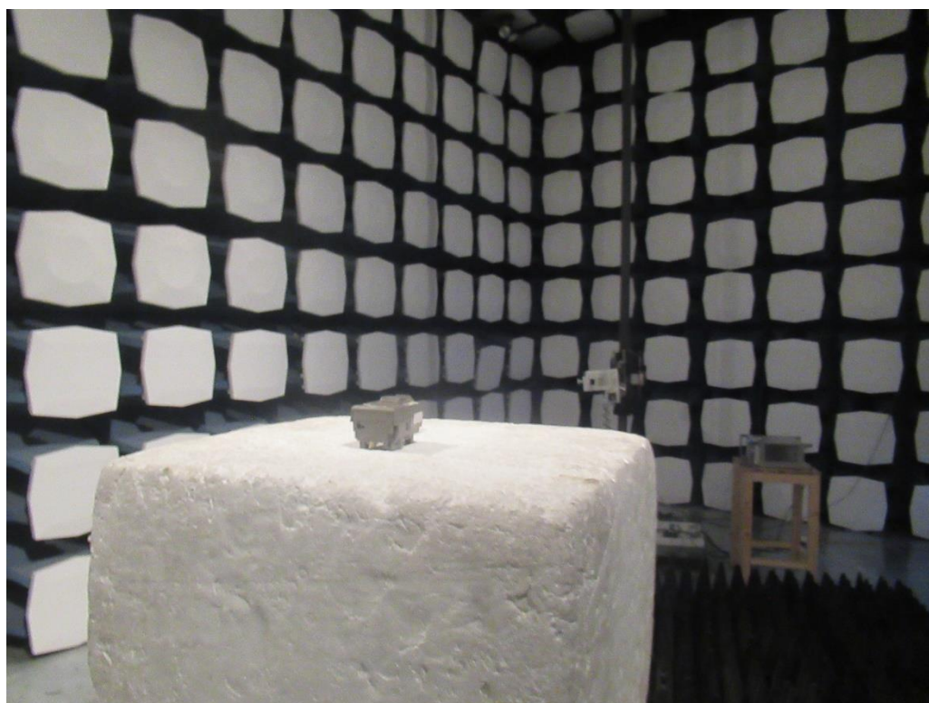
Picture 1 Radiated Emission Test Setup
