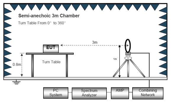
(B) Radiated Emission Test-Up Frequency 30MHz~1GHz
