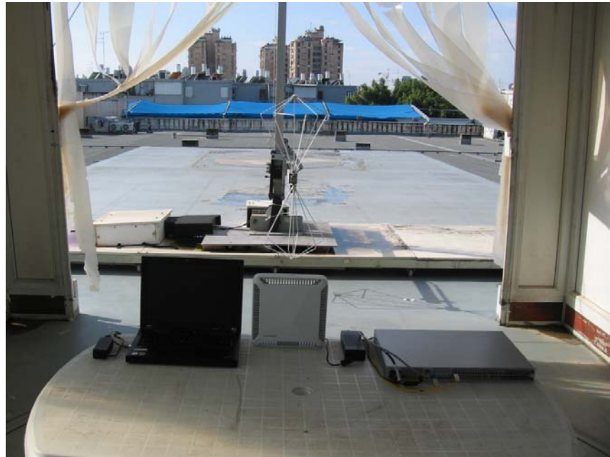
Figure 5. Radiated Emission Test, 30-200MHz
