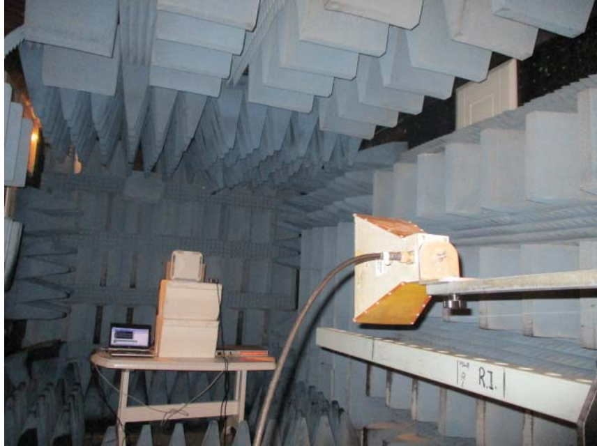
Figure 7. Radiated Emission Test, 1-18GHz
