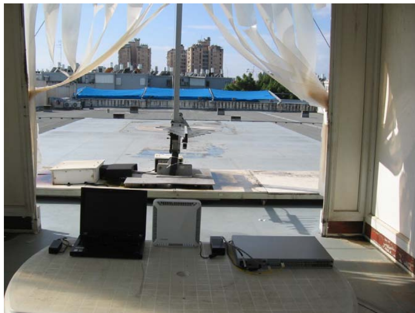
Figure 6. Radiated Emission Test, 200-1000MHz
