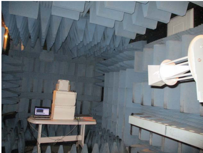
Figure 8. Radiated Emission Test, 18-26.5GHz
