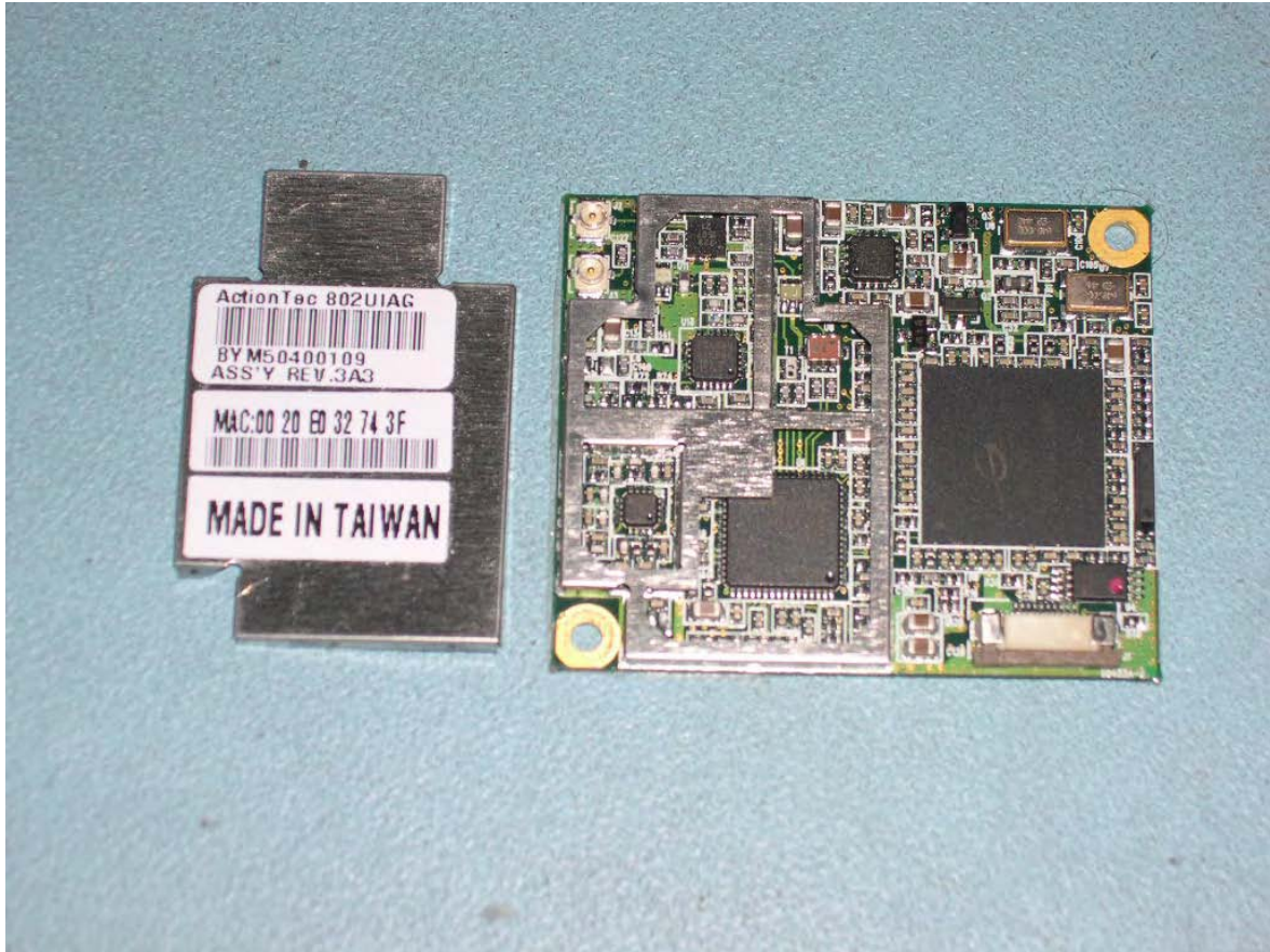
Top of Radio Card with Shield Removed
