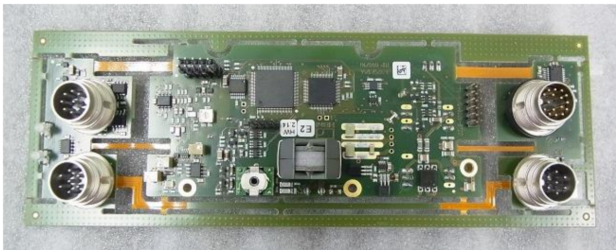
Picture 34: PCB stator rear side
