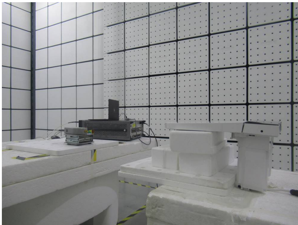
Photograph 7: Set-up photo for Radiated Spurious Emission, 75GHz ~ 100GHz
