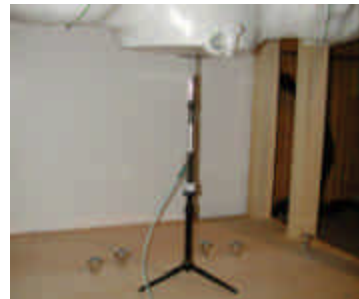
Figure 12.1 Dipole Validation Test Setup
