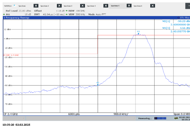
Figure 7.7-14: Conducted non-restricted band edge spurious emissions at 2400 MHz, Low ch.
