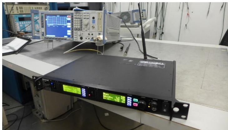
Figure 1: Test setup for Maximum Radiated Output
