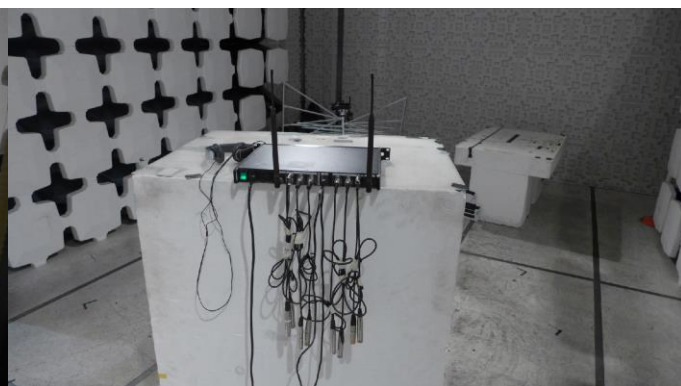
Figure 2: P10T Transmitter Test Setup
