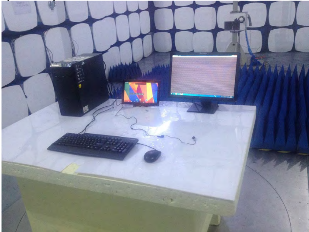
Photograph 3: Set-up for Radiated Emission of above 1GHz
