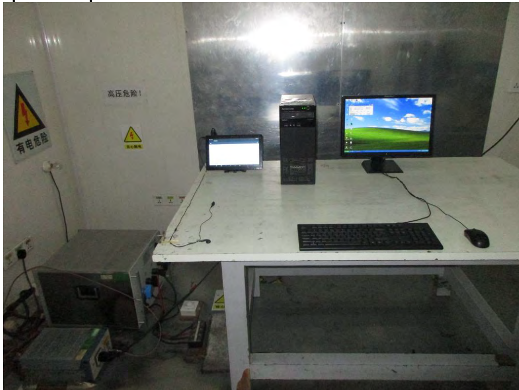
Photograph 2: Set-up for Radiated Emission of below 1GHz
