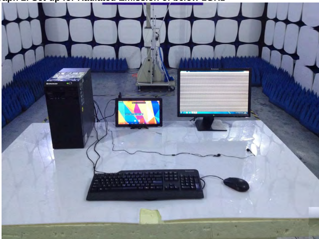
Photograph 2: Set-up for Radiated Emission of below 1GHz
