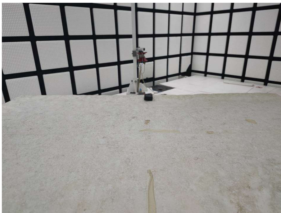
Radiated spurious emission Test Setup-2(Above 1GHz)
