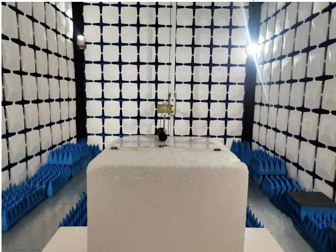
Above 1GHz for radiated emission test setup
