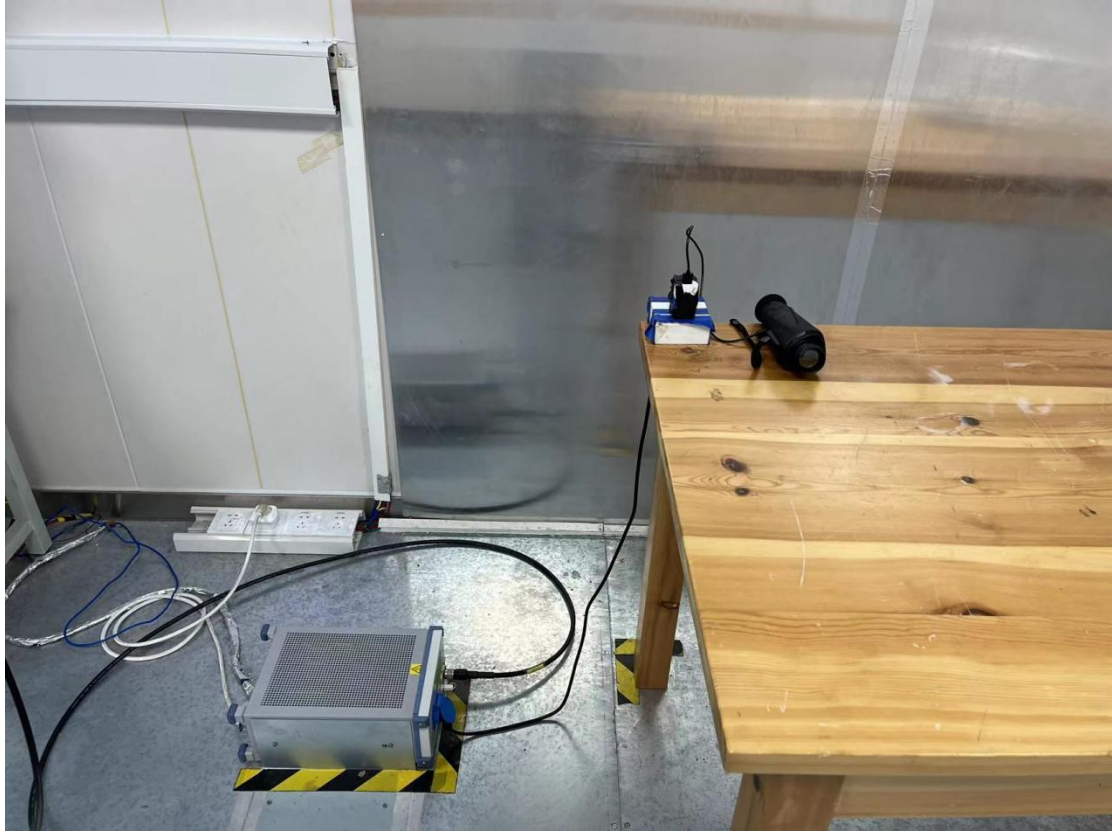
Conducted emission test setup
