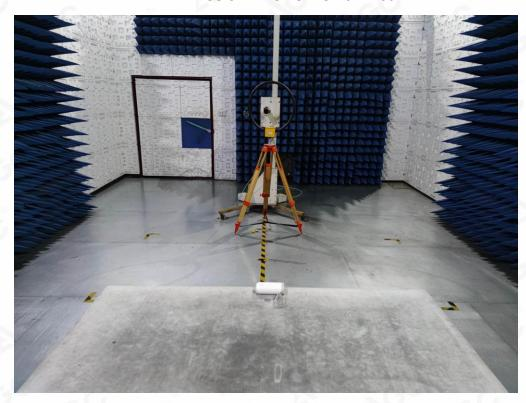
RADIATED EMISSION TEST SETUP BELOW 1GHz
