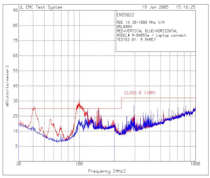
Radiated Disturbance Emissions - 30 to 1000 MHz Electric Field
