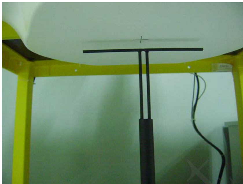
Setup Photo of Dipole Antenna
