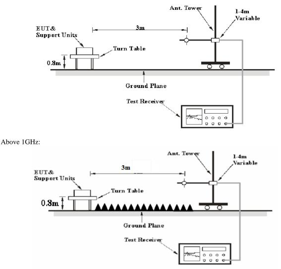
The radiated emission below 1GHz tests were performed in the 10 meters chamber test site, above 1GHz tests were performed in the 3 meters chamber test site B, using the setup accordance with the ANSI C63.4-2014. The specification used was the FCC Part 15.109 Class B limits.
