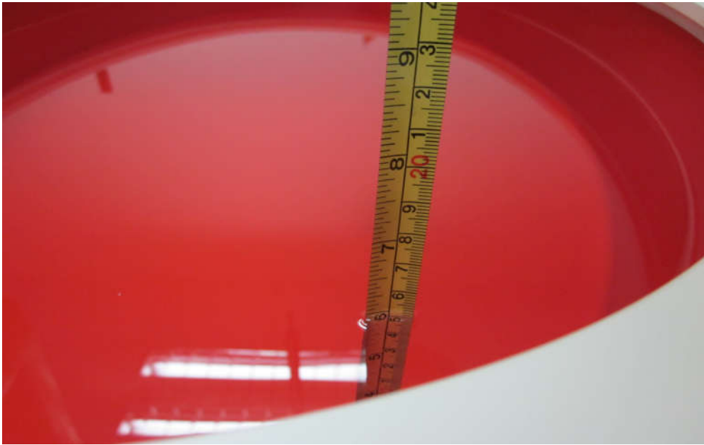
Figure 4.4: Liquid depth in the Flat Phantom
