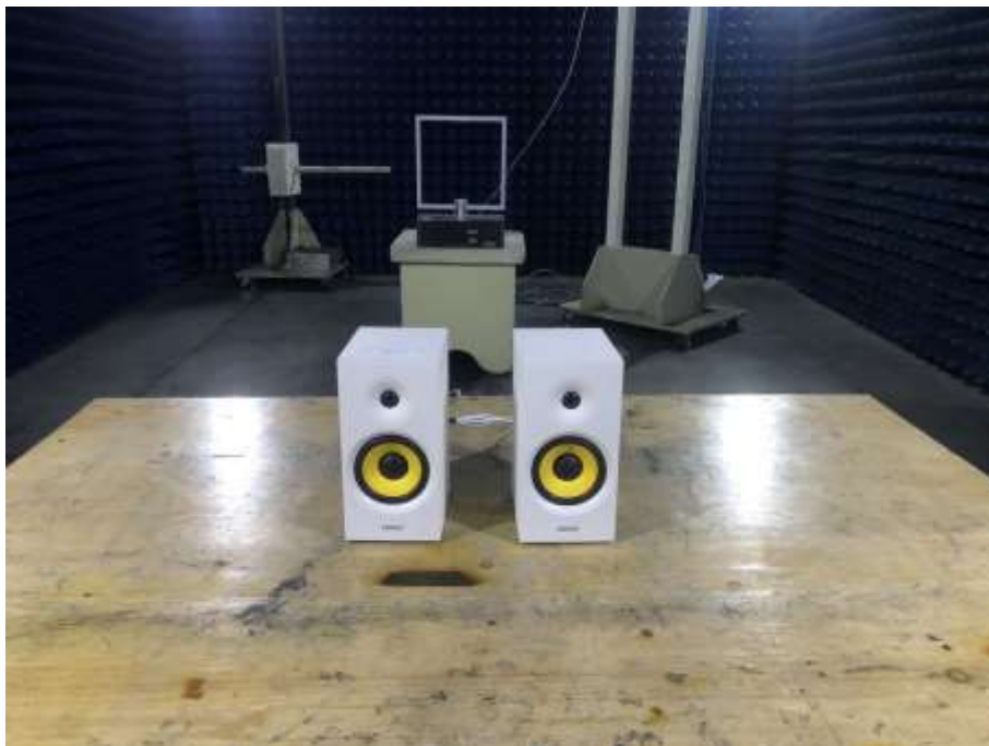
Photograph 2: Set-up for Radiated Spurious Emission, 9KHz - 30MHz
