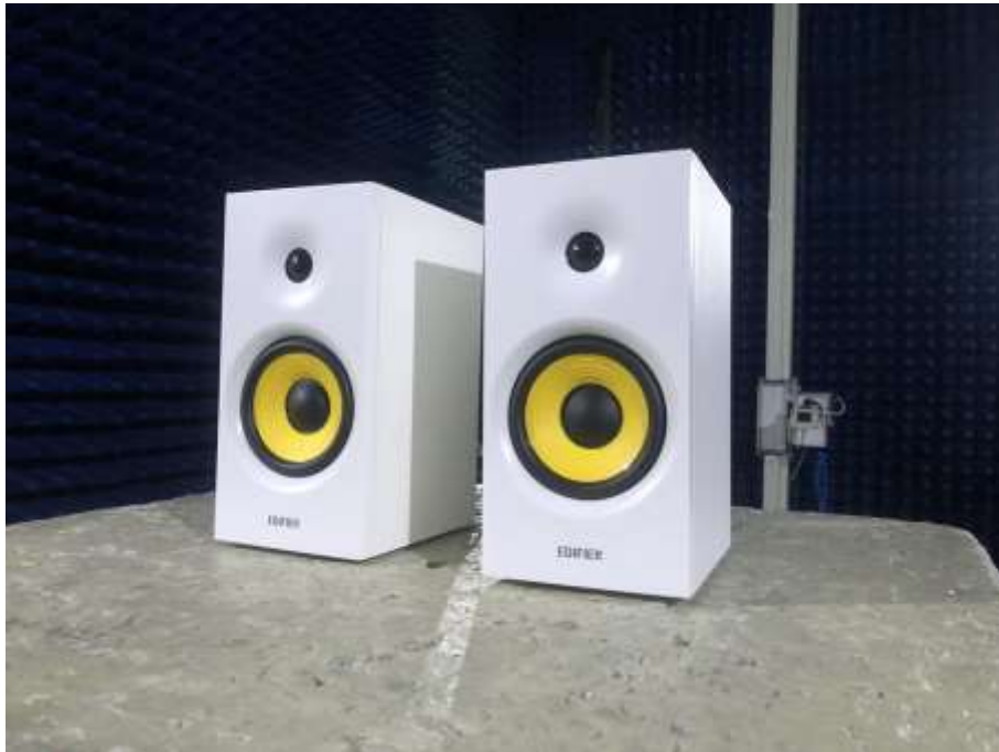
Photograph 5: Set-up for Radiated Spurious Emission, 18GHz - 26.5GHz
