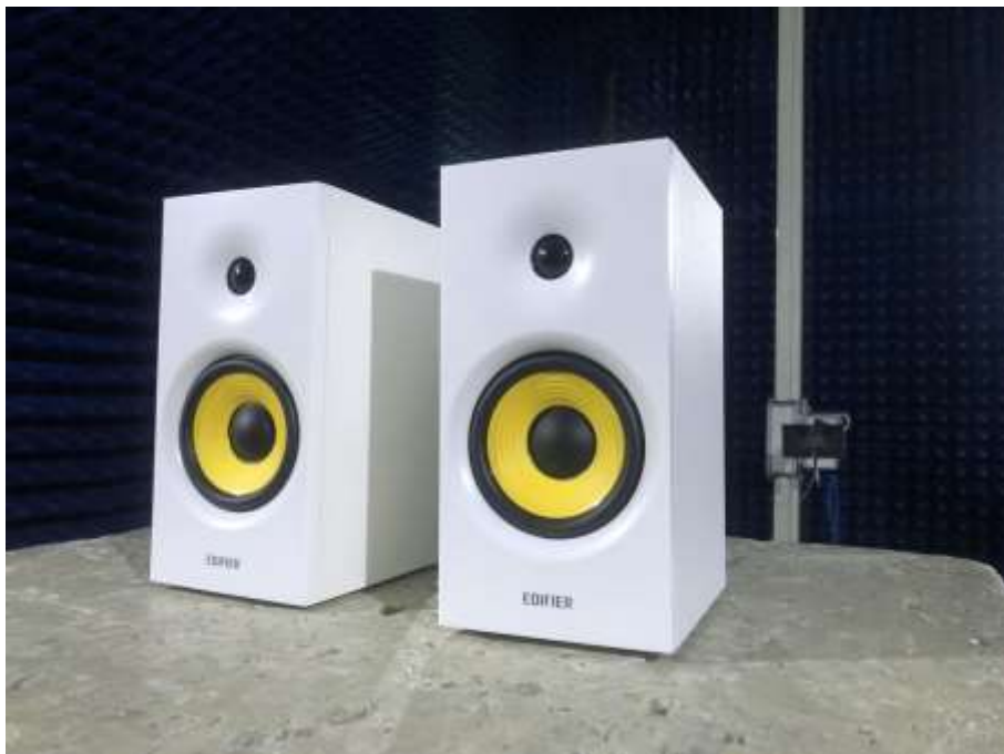
Photograph 4: Set-up for Radiated Spurious Emission, 1GHz - 18GHz
