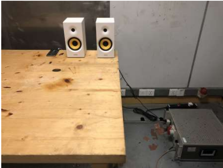
Photograph 1: Set-up for Conducted Emission on AC Mains
