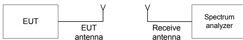
Figure 7.2.1 Occupied bandwidth test setup
