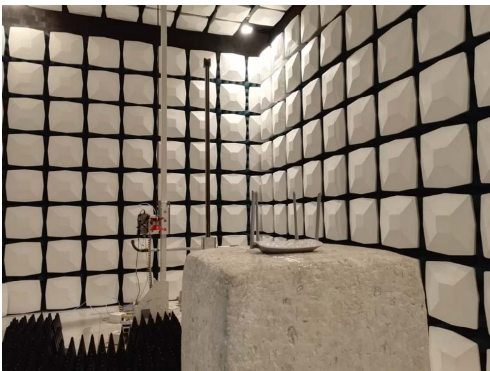
Description: Radiated Emission Test Setup for 1~18GHz
