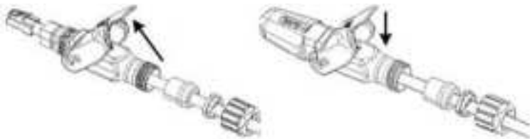
Figure 35: Align RJ45 into Holder
