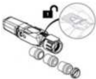
Figure 41: Open Housing Lock
