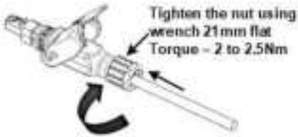
Figure 38: Tighten Gland Nut
