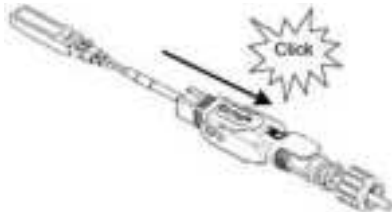
Figure 21: Holder into Housing Base
