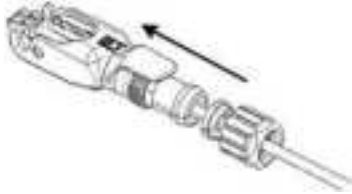
Figure 18: Pass Cable thru Housing
