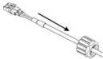
Figure 15: Gland Nut on Cable
