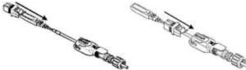
Figure 20: Insert Holder over the Transceiver
