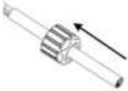
Figure 43: Insert Gland Nut
