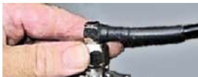
Figure 53: Connecting Antenna RF Cable
