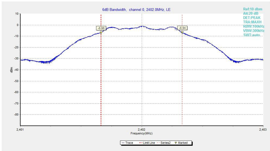
Fig.20. 6dB Bandwidth: GFSK, 2402 MHz
