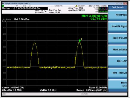
EIRP PSD=-32.774+1+5=-26.774dBm/MHz, attenuation of Cable and Splitter is 5dB, Antenna gain is 1dBi.
