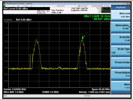
EIRP PSD=-26.937+1+5=-20.937dBm/MHz, attenuation of Cable and Splitter is 5dB, Antenna gain is 1dBi.
