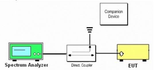
End User Device as UUT, the companion device is certified CBRS (FCC ID: 2AG32PBS31010)
