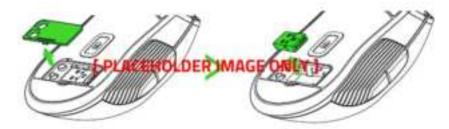
2. Reattach the compartment cover and insert the wireless USB dongle into the USB port of your PC.
