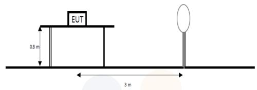
The diagram below shows the test setup that is utilized to make the measurements for emission from 30 № to 1 № emissions.
