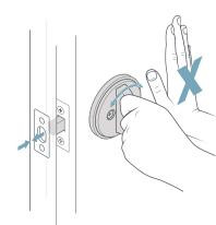
02 Disassemble your lock and keep pieces. Unscrew the lock housing, the deadbolt, and the strike plate. Store the deadbolt and strike plate in the Level box.
