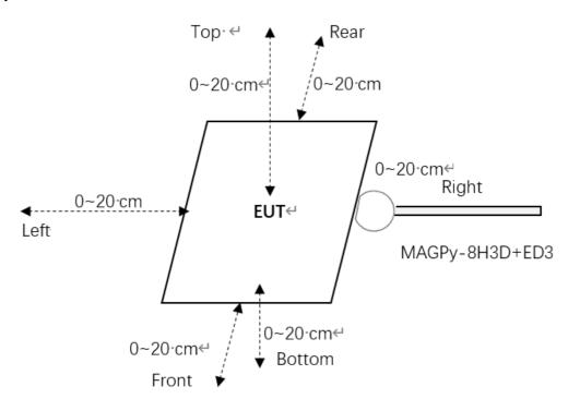
Note: tips mode of the test probe is used for 0cm measurement.
