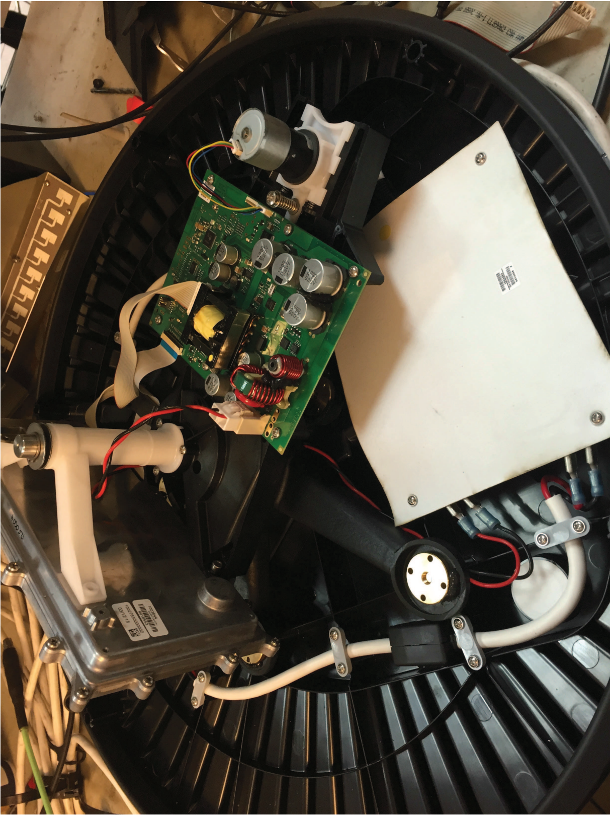
Figure 1 – Radar – dome cover removed
