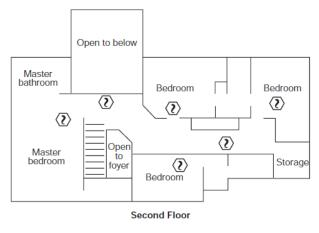
Example of smoke alarm requirements for large house with multi-floor spaces. (Source: NFPA 72, National Fire Alarm and Signaling Code Handbook, 2013.)
