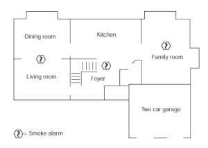
Example of spacing criterion of one or more smoke alarms for every 500 ft<sup>2</sup> (46 m<sup>2</sup>) of interior floor area on every floor greater than 1000 ft<sup>2</sup> (93 m<sup>2</sup>). (Source: NFPA 72, National Fire Alarm and Signaling Code Handbook, 2013.)
