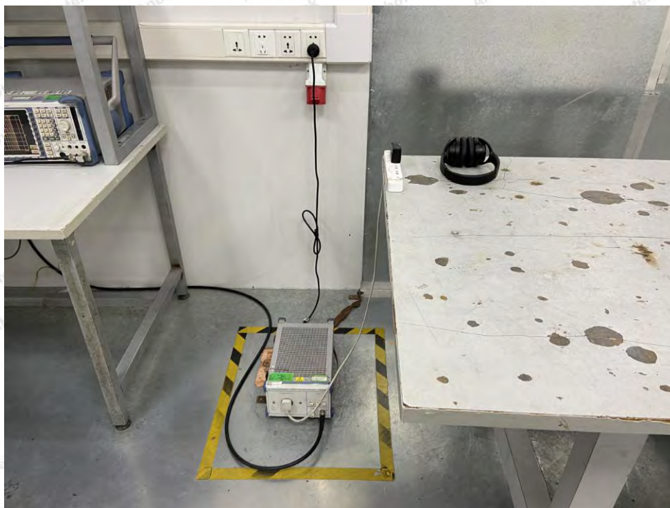
Photo of Conducted Emission Measurement
