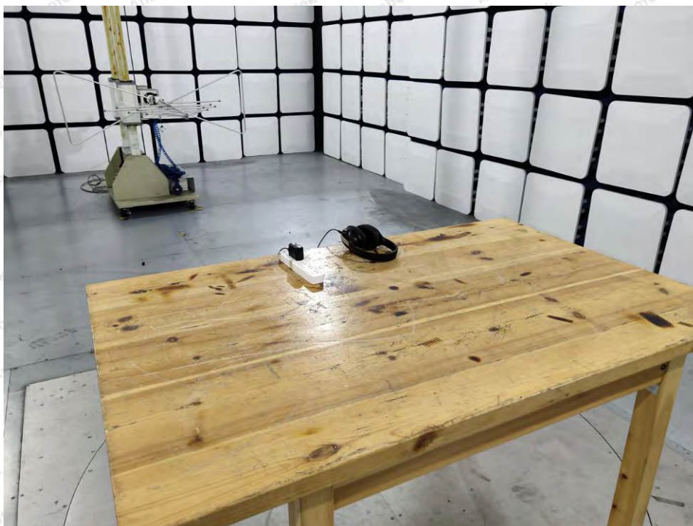
Photo of Radiation Emission Test
