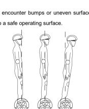
Move Backward Stop Move Forward Dismounting your device can be one of the easiest steps, yet when done incorrectly,
