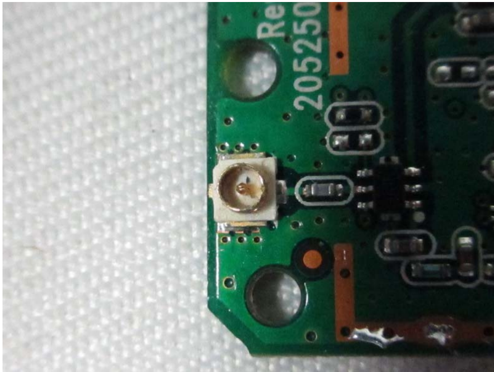
RF module antenna connector
