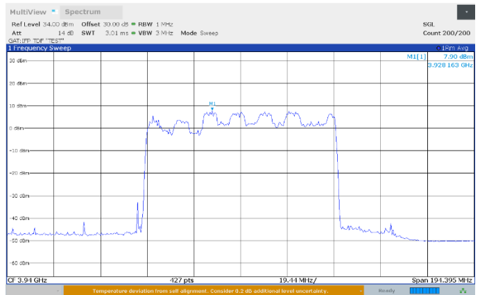
Average PSD, TX: 3940 MHz, BW: 80MHz, MOD: 16QAM
