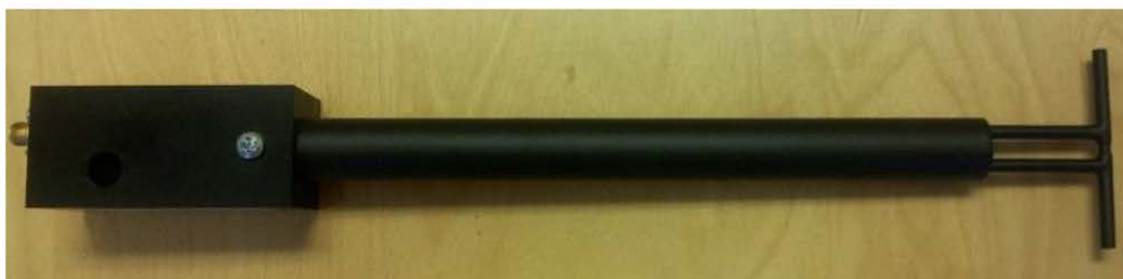
Figure 1 – MVG COMOSAR Validation Dipole
