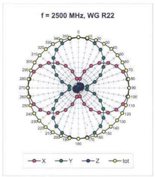
Receiving Pattern ( $\phi$ ),  $\vartheta = 0^{\circ}$
