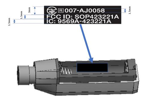
FCC ID and IC No are sure to be recognized by users at the first use as it requires the battery insertion before use.
