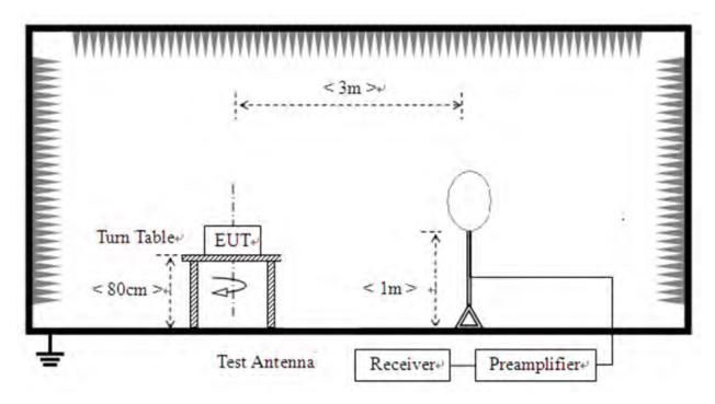
2) For radiated emissions from 30MHz to1GHz
