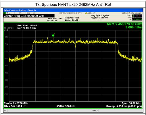
Tx. Spurious NVNT ax20 2462MHz Ant1 Emission
