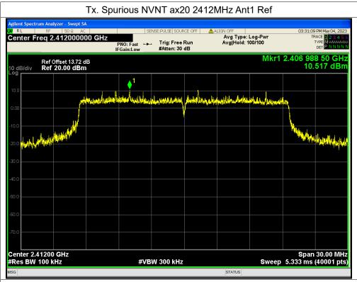
Tx. Spurious NVNT ax20 2412MHz Ant1 Emission
