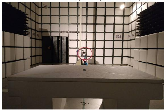
Radiated Emission Set up Photos (Below 1GHz, 3M)
