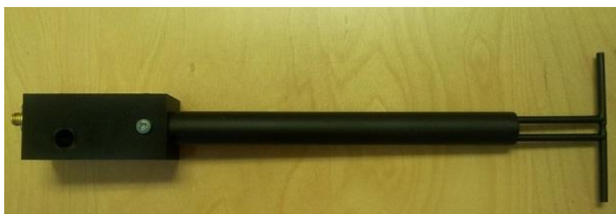
Figure 1 – MVG COMOSAR Validation Dipole
