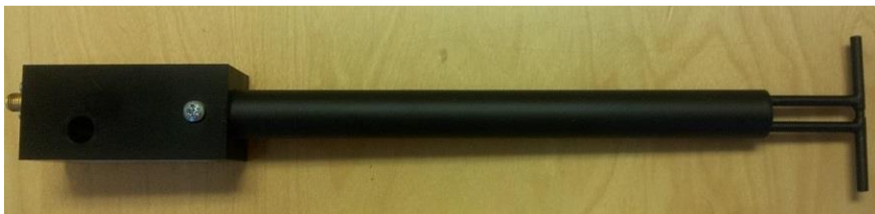
Figure 1 – MVG COMOSAR Validation Dipole
