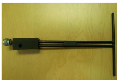
Figure 1 – MVG COMOSAR Validation Dipole
